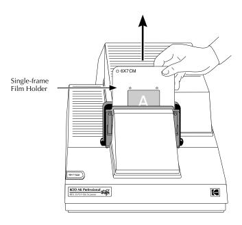
C. If the single-frame holder adapter is not in the Scanner, put it in place in the Scanner. Do so by holding it in the orientation shown below with the slots (at the left and right of the adapter) facing forward, and then slide the slots all the way down over the edges of the front of the metal frame in the Scanner.
